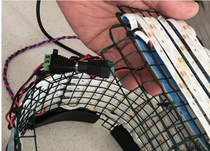
Clip the top back into place, plug in the new Male connector.
