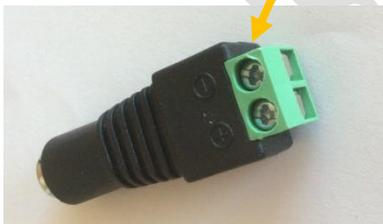
Take the red positive wire that you have just released and the red positive wire from the cable you have threaded down. Squash them firmly together (it helps to roll them between your fingers to get a tight wire) and insert into the positive side of the above connector. Screw them tightly in place.
