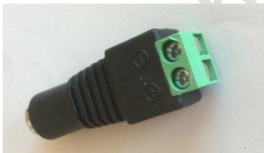
Match the (+) on the strip with the (+) on the connector. Thread the wire in, pushing it as far into the slot as possible. Using your small Phillips head screwdriver, screw down and you should find that your wires are securely attached. Give them a gentle tug to see if you can pull them out. If they resist a gentle tug, you have a secure connection.
